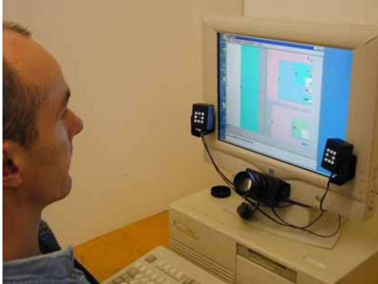
Using Dasher with an eyetracker
