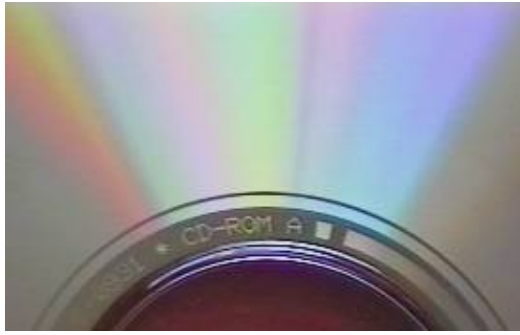
Figure 2: The grooves on a CD are only 0.5 micro-metres wide and make a good diffraction grating, resulting in coloured interference patterns.
