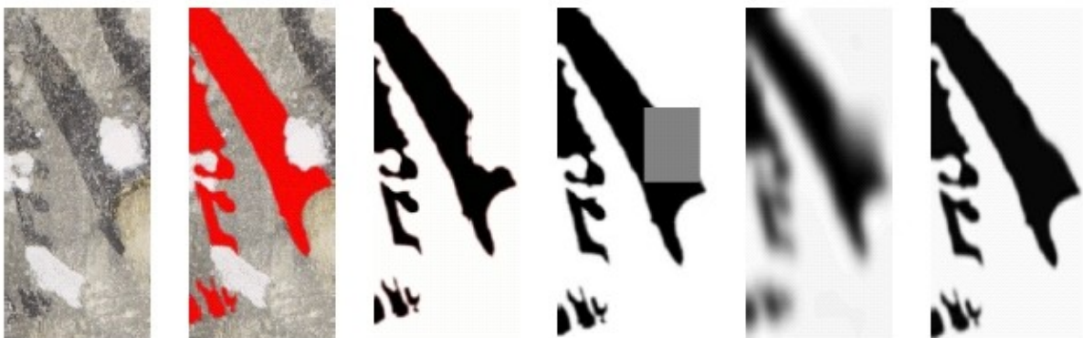
Figure 10: A specific structure in the fresco is selected and then reconstructed using Cahn–Hilliard inpainting for black and white images. From left to right: the original image; the relevant structure is identified; the structure is binarised (turned into a black and white image); the missing domain is identified (grey rectangle); the image structure is diffused into the missing domain, the structure is sharpened.
